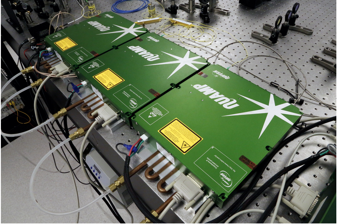
Figure 6.5: Photograph of the three Nufern NUA-1064-PB-0015-B3 fibre amplifiers used in the amplifier-compatible OPA.
